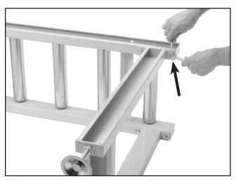
**Figure 11.** Attaching stand leg/foot assembly to roller table.
